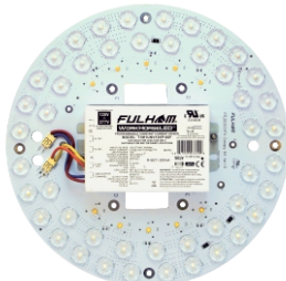
LED Engine (LED driver comes pre installed)
