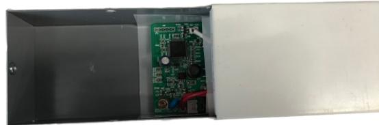
Re-connect the battery connector and place all wires back into the battery cover
