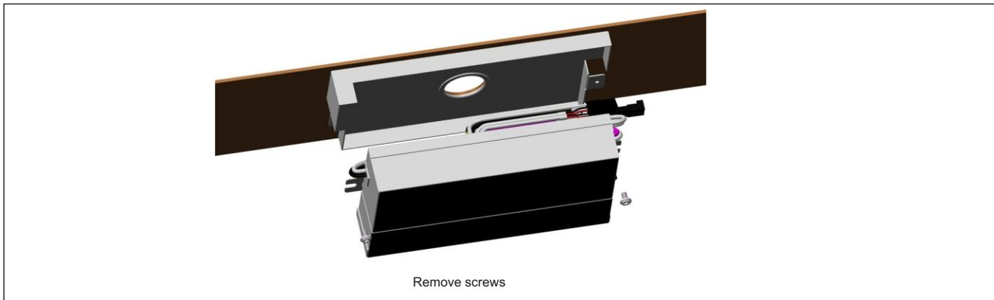
**STEP 1:** Remove the LED driver from the bottom feed cover
