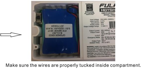
Make sure the wires are properly tucked inside compartment.
