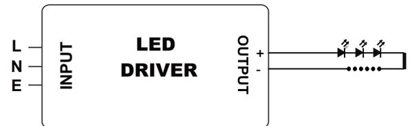
**Installation Instructions:** Keep proper ventilation around the LED Driver and do not stack any object on it. Also a 10-15 cm clearance must be kept when the adjacent device is a heat source. Do not exceed the declared Hot spot temperature(Tc max) under any circumstances.
