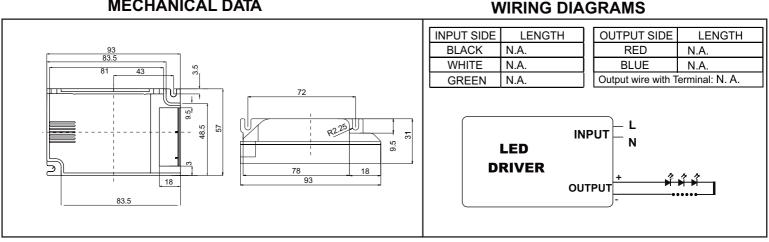
Installation Instructions: Keep proper ventilation around the LED Driver and do not stack any object on it. Also a 10-15 cm clearance must be kept when the adjacent device is a heat source. Do not exceed the declared Hot spot temperature(Tc max) under any circumstances.
