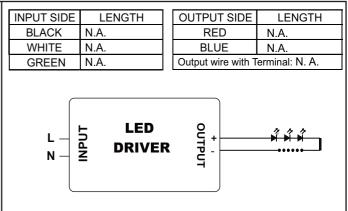
Installation Instructions: Keep proper ventilation around the LED Driver and do not stack any object on it. Also a 10-15 cm clearance must be kept when the adjacent device is a heat source. Do not exceed the declared Hot spot temperature(Tc max) under any circumstances.
