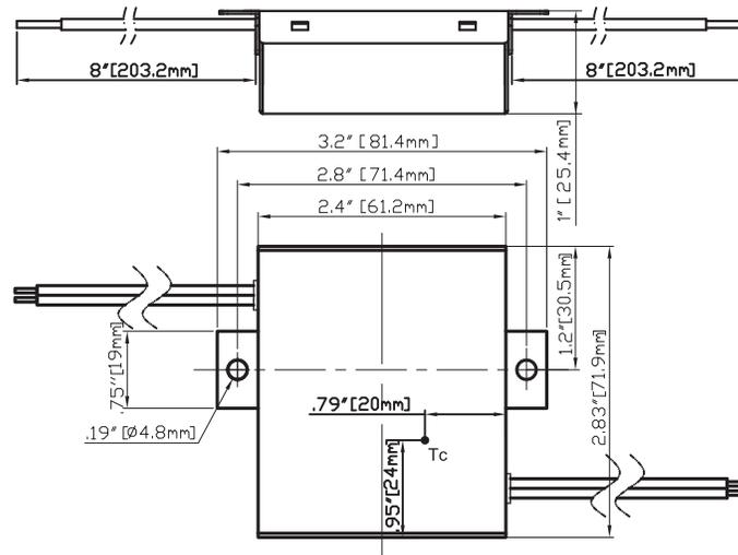
Where : L = Length, W = Width, H = Height, Tolerance=±0.02"
