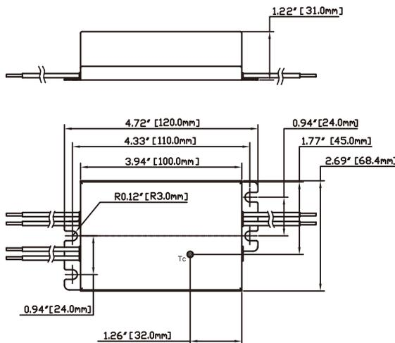
Where : L = Length, W = Width, H = Height, Tolerance=±0.02"
