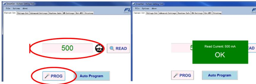
The above shows the “PROGRAM” function in the software which is used to set an appropriate output current on the driver. This can be used for single or small batch programming. After typing in the appropriate current select the “PROG” button to program/set the drivers output current.
