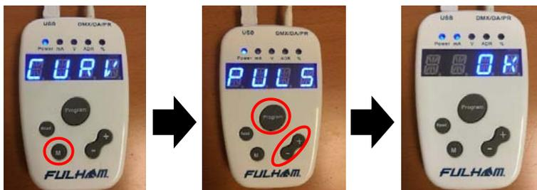
While in full mode, use the **“M”** button to cycle through the menu options until the **“CURV”** option is displayed. Next use the **“+”/“-”** buttons to select the **“PULS”** option then press the **“PROGRAM”** button, **“OK”** will flash on the screen indicating the Pulse Dim protocol has now been set on the driver.
