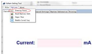
Under the Options setting the user can select the Dimming Curve option in the dropdown menu. This option allows the creation of a custom dimming curve. The user can then select certain minimum and maximum levels to dim to, as well as enable/disable dim to off.
