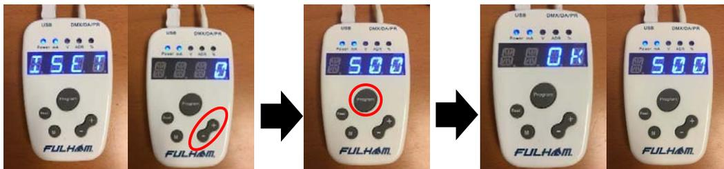
To program a Current or Voltage (“ISET” or “VSET” must be selected), use the “+”/“-” buttons to dial in the appropriate value, then press the “PROGRAM” button. If successful, the display will flash “OK” followed by the programmed current. If needed you can verify that the current has been set by re-reading the value, which can be done by again pressing the “READ” button (Refer to “TPSB-100/E - Simple Mode - Reading”).
