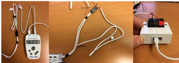
Programmable drivers with connectors on their output can be programmed using the mating connector cable. If the drivers mating output harness is plugged in, then they can be programmed using the wires labeled **R-SET/PRG/NTC** by plugging them into the Red (+) and Black (-) quick release connectors located on the top of the wire block adapter. The polarity of the program wires are as follows; Orange Wire (+), Yellow wire (-), Purple Wire (+), Grey Wire (-), Red Wire (+), Black Wire (-).
