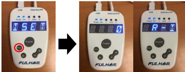
Pressing the “READ” button will allow reading of the programmed parameters for either “ISET” (Current) or “VSET” (Voltage). After pressing the read button, the screen will display the value that is currently programmed to the driver followed by “R – I” (Current Read) displayed on the screen.
