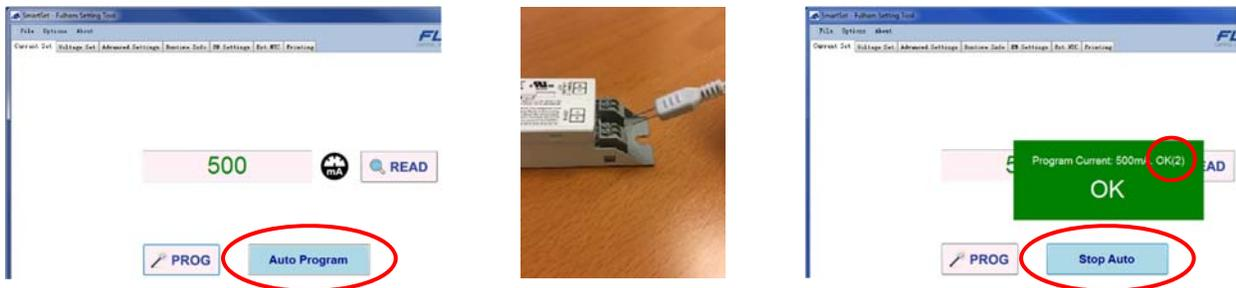
The above shows the “Auto Program” function in the software. This can be used for large batch programming of drivers that will have the same programmed current. After each program, all that is needed is to insert / connect to the port / leads of the TPSB-100/E. The software will keep a count of the number of drivers programmed. To stop the auto programming simply press the “Stop Auto” button.
