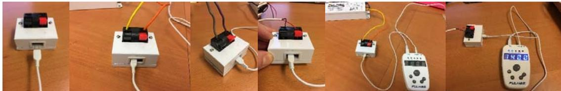
Programmable drivers with wires can be programmed using the wire block adapter. Insert either the larger or smaller pitched fork cable into the back of the adapter. Ensure that proper polarity is established. Next insert the wires labeled **R-SET/PRG/NTC** into the Red (+) and Black (-) quick release connectors located on the top of the adapter. The polarity of the programming wires are as follows; Orange Wire (+), Yellow wire (-), Purple Wire (+), Grey Wire (-), Red Wire (+), Black Wire (-).
