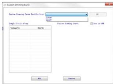
The software will generate a dimming curve based on the input set by either selecting one of the custom dimming curve profiles in the pulldown menu or entering the voltage with dimming percentage on the table to the left. A minimum of 2 points are required to generate a custom dimming curve. This allows Fulham's programmable driver to match the dimming curve of other driver suppliers.
