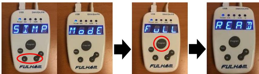
Under “FULL MODE” you will be able access advance features. To enter full mode press and hold the “M” and “-” buttons simultaneously until the screen flashes “FULL”/ “MODE”, immediately press the “PROGRAM” button three times. The screen will display “READ” indicating that it’s reading the advance parameters of the driver.
