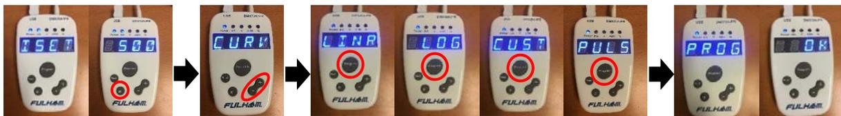
While in **"FULL MODE"** applicable drivers will have the ability to change the dimming profile to either Linear **"LINR"**, Logarithmic **"LOG"**, Custom **"CUST"** or Pulse **"PULS"**. Use the **"M"** button to cycle through the various programming options. Once **"CURV"** is displayed use the **"+"**/**"-"** buttons to dial in the appropriate dim profile, then press the **"PROGRAM"** button. The screen will flash **"PROG"**/**"OK"** indicating the desired profile has been programmed.
