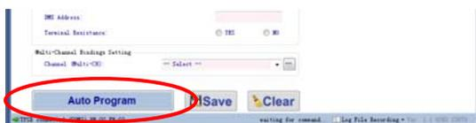
With this feature, auto programming of the advanced settings is done once the programming port / leads are connected to the TPSB-100/E. All the units are set to the appropriate current, and all settings from the Advanced Settings tab are transmitted to every unit. A count of the number of drivers that have been programmed is kept.
