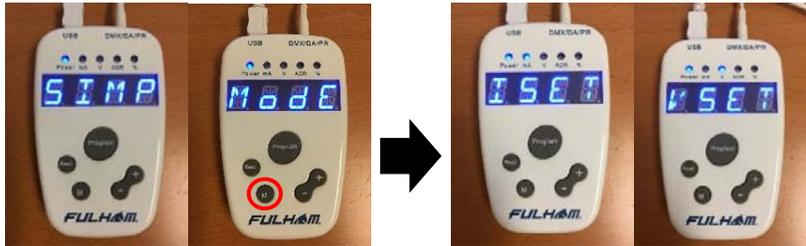
When first powered up the Setting Controller defaults to Simple Mode and will toggle a display of “SIMP” / “MODE”. While in simple mode the parameters you can program are limited to either “ISET” (Current) or “VSET” (Voltage). Pressing the “M” button will allow you to cycle through the programming options of either voltage or current.
