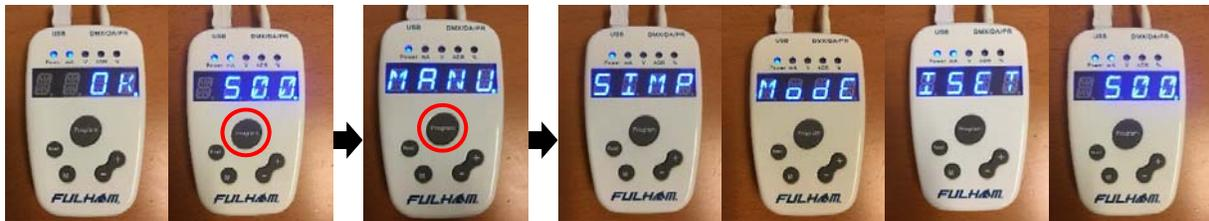
To exit the auto program feature press and hold the “PROGRAM” button. When you see “MANU.” displayed on the screen, immediately press the “PROGRAM” button three times. “SIMP”/“MODE” will quickly flash on the screen followed by either “ISET” or “VSET” and its value being displayed on the screen.
