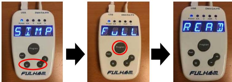
First the setting controller must be in **“FULL MODE”** to access the advance features. To enter full mode press and hold the **“M”** and **“-”** buttons simultaneously until the screen flashes **“FULL MODE”**, immediately after press the **“Program”** button three times. The screen will display **“READ”** indicating that it’s reading the advance parameters of the driver.
