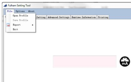
Under the File pulldown menu, the user can access the “Open Profile” or “Save Profile” options. Once a driver has been programmed to the setting needed, the profile can be saved for later access to program more drivers to these specific settings.
