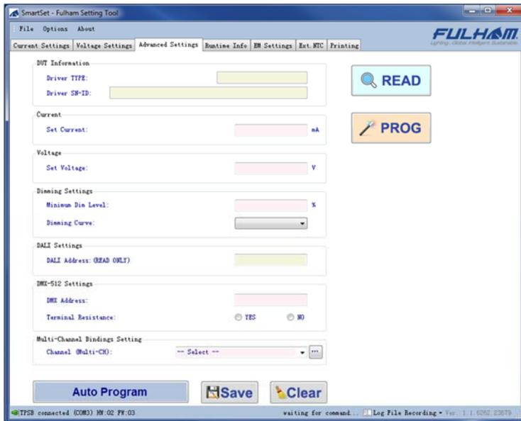
The Advanced Setting tab also gives the user the ability to set different parameters, such as dim levels, dimming curves (linear, logarithmic or custom), and DMX settings, and even to group multiple channels on supporting drivers.
