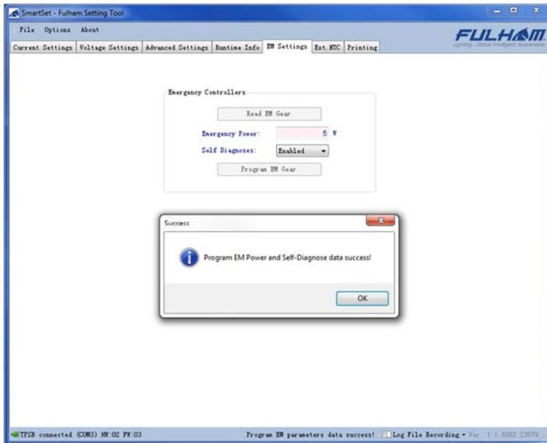
Under the EM Settings tab for applicable products you will be able to read existing emergency characteristics as well as program additional emergency features. Such features as setting/programming the emergency power, as well as the ability to Enable/Disable Self-Diagnostics.
