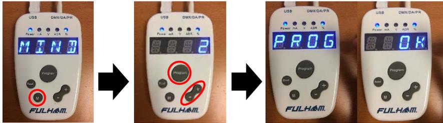
While in **“FULL MODE”** applicable drivers will have the ability to change the minimum dim level percentage. Use the **“M”** button to cycle through the various programming options. Once **“MIND”** is displayed use the **“+”/“-”** buttons to dial in the appropriate percentage, then press the **“PROGRAM”** button. The screen will flash **“PROG”/“OK”** indicating the desired profile has been programmed.
