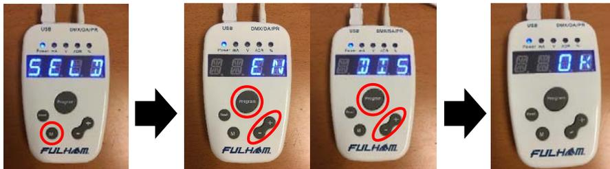
While in **"FULL MODE"** applicable drivers will have the ability to enable or disable the Self-Diagnostic feature. Use the **"M"** button to cycle through the various programming options. Once **"SELD"** is displayed use the **"+"**/**"-"** buttons to dial in either **"EN"** (Enable Self-Diagnostics) or **"DIS"** (Disable Self-Diagnostics), then press the **"PROGRAM"** button. The screen will flash **"OK"** indicating the desired option has been programmed.
