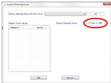
The dim to off feature allows you to dim down below a certain point where the driver turns off and then turns back on once you've got back up past that point.
