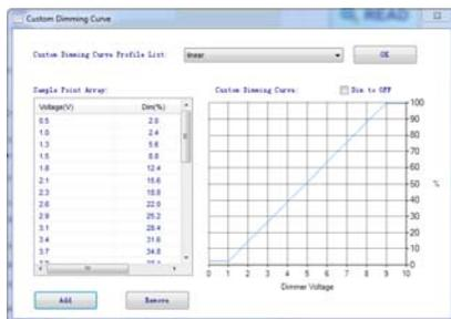
The image above shows a plot of what the dimming curve looks like and the breakdown of the voltage assigned to the percentage of dimming.
