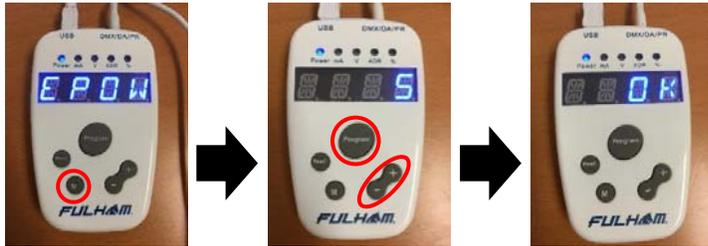
While in **"FULL MODE"** applicable drivers will have the ability to program emergency power. Use the **"M"** button to cycle through the various programming options. Once **"EPOW"** is displayed use the **"+"**/**"-"** buttons to dial in the appropriate value, then press the **"PROGRAM"** button. The screen will flash **"OK"** indicating the desired power has been programmed.
