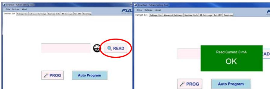
The above shows the “READ” function in the software which is used to determine what current the driver is programmed to.
