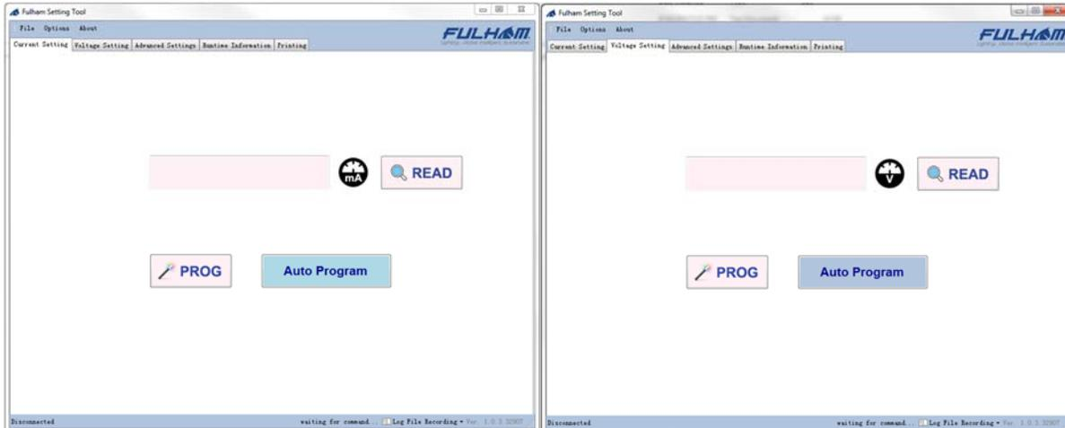
Using either the Voltage or Current tab in the Setting Tool interface the user can easily input the desired values. Depending on the driver, for a constant current application the user can program the desired output current dependent on the minimum and maximum current settings of the driver (refer to the specification sheet of driver for further information).
