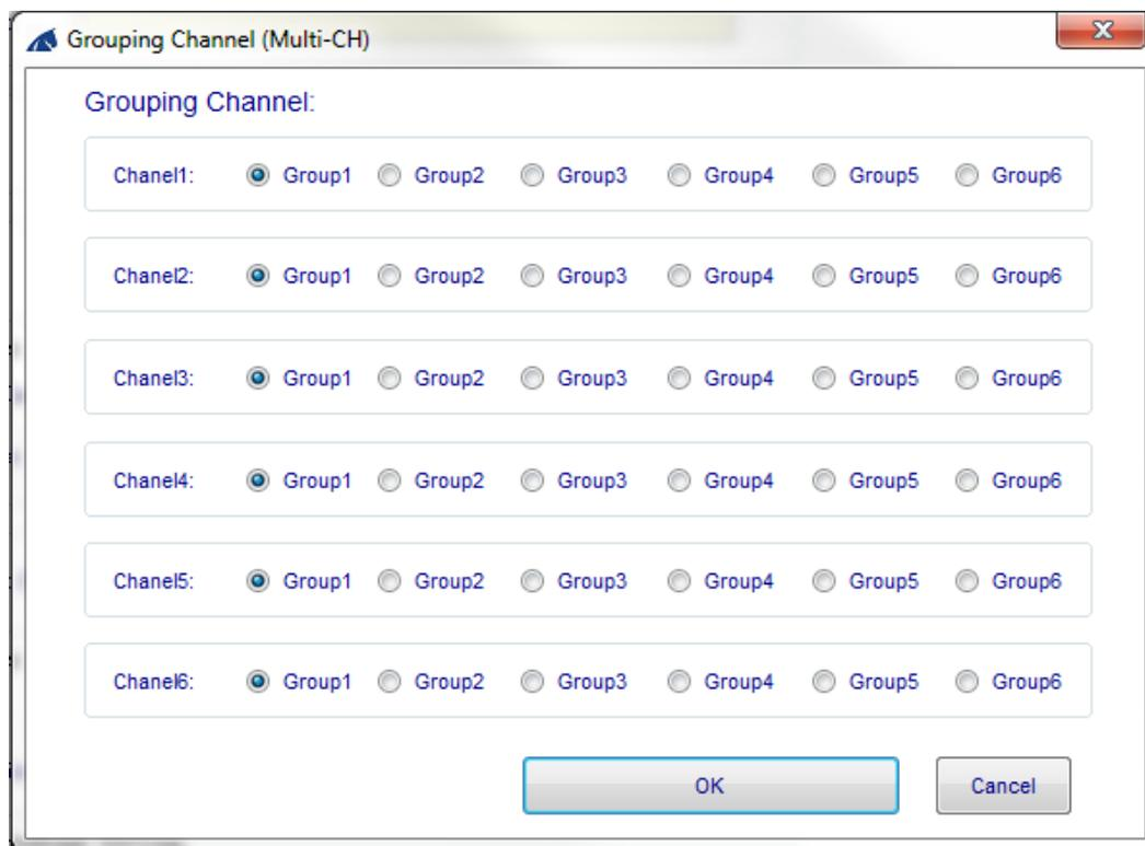
With DMX drivers, users will have the ability to group different output channels together.
