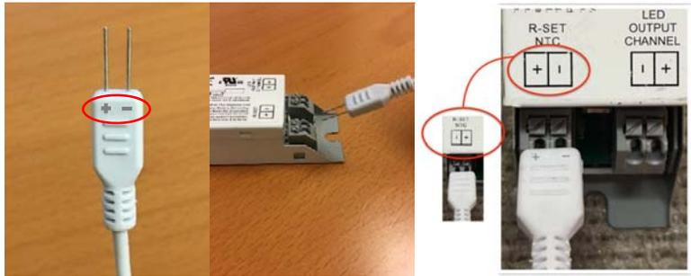
Programmable drivers with push in connectors can be programmed using either the larger or smaller pitch fork cables. Simply insert the forks directly into the connectors labeled **R-SET/PRG/NTC**, ensure that proper polarity is established otherwise an error code will be displayed.
