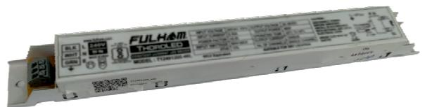
**Installation Instructions:** Keep proper ventilation around the LED Driver and do not stack any object on it. Also a 10-15 cm clearance must be kept when the adjacent device is a heat source. Do not exceed the declared Hot spot temperature(Tc max) under any circumstances.
